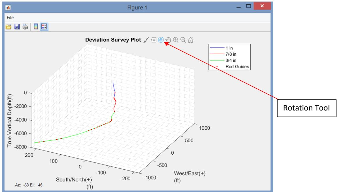
**Figure 67 – Rotation capability for 3D survey plots**
