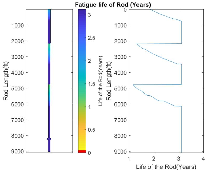
**Figure 38 Fatigue life of Rod**
