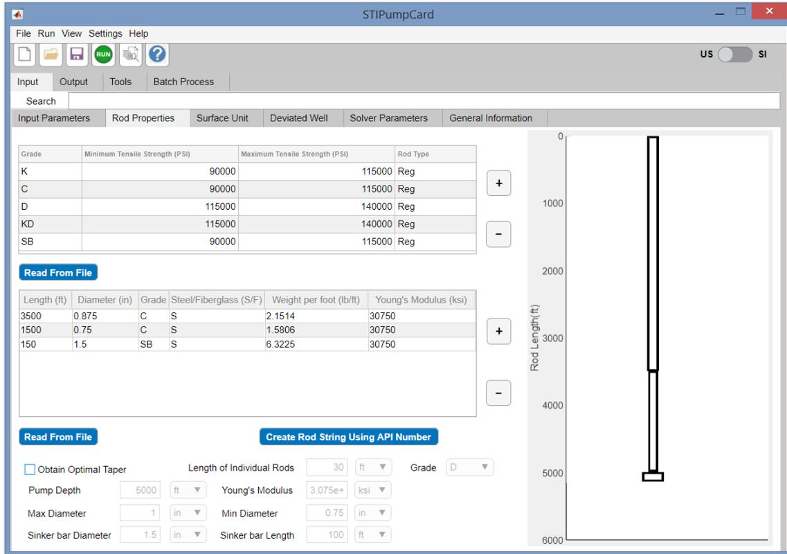
Figure 10 - Rod properties Tab
