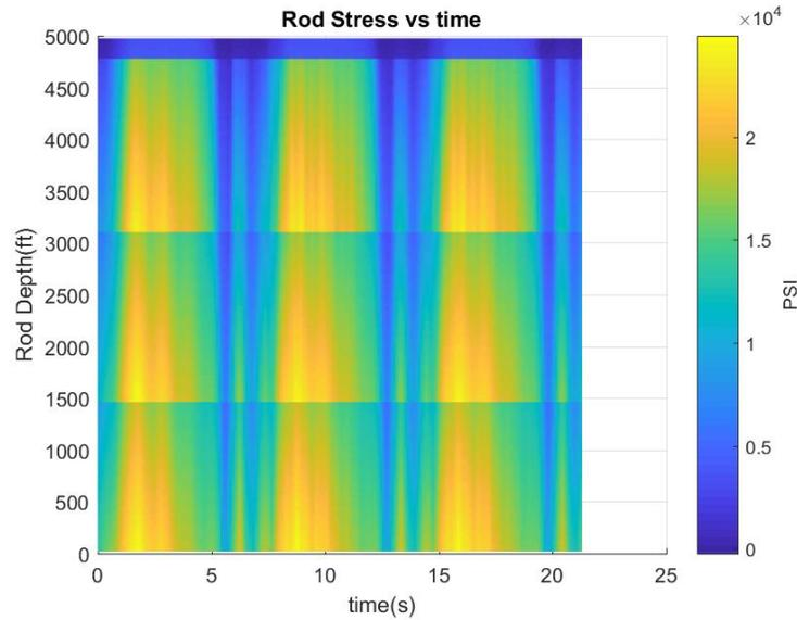
Figure 36 - Rod Stress vs. Time
