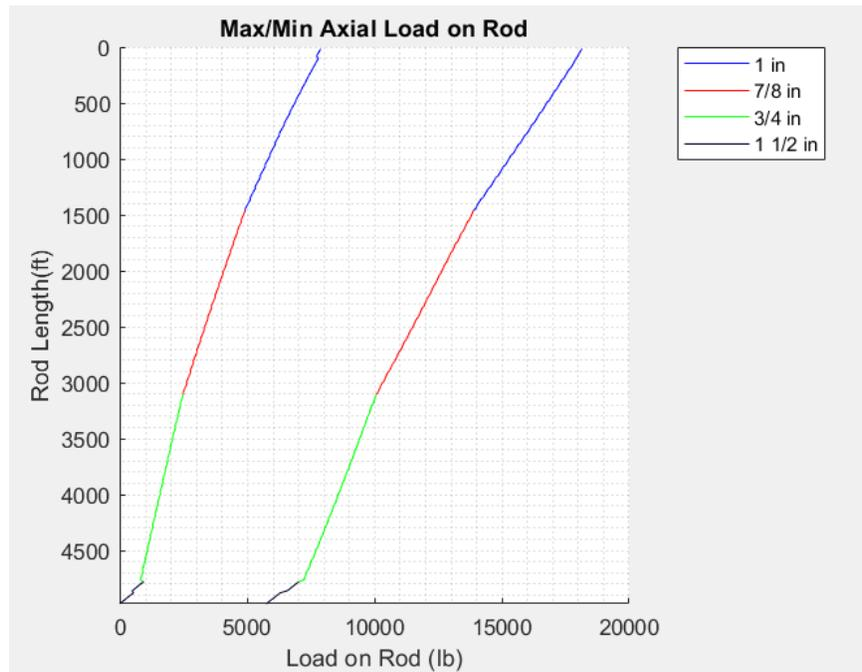
Figure 37 - Axial Load on Rod
