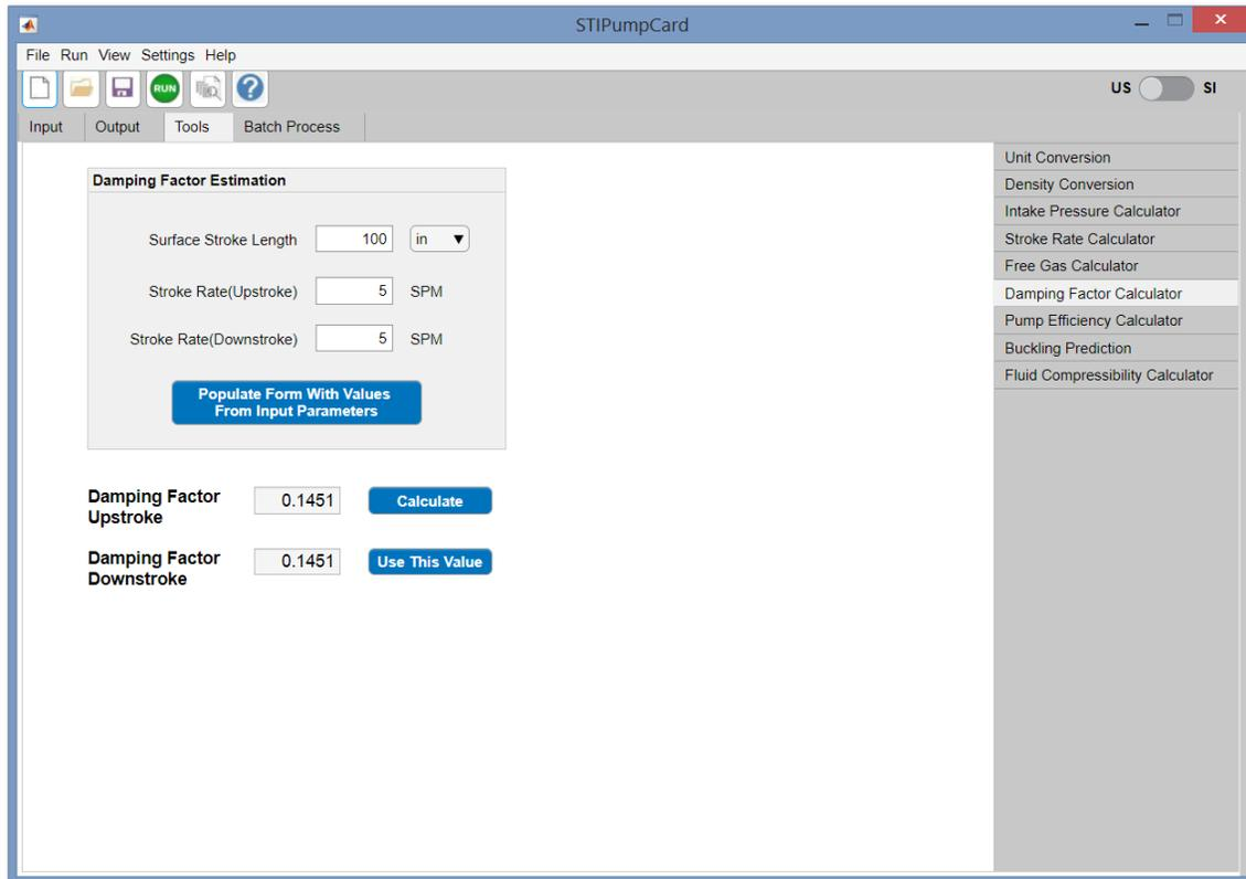
Figure 61 - Damping Factor Calculation Panel
