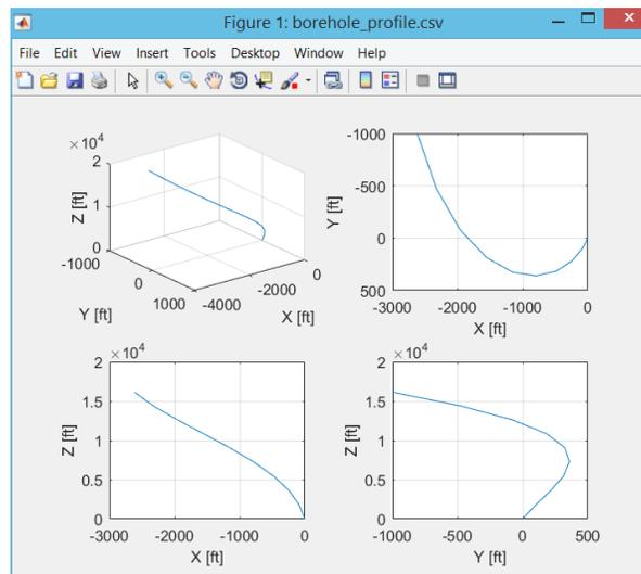
**Figure 28 - Borehole Profile Plot Sample**
