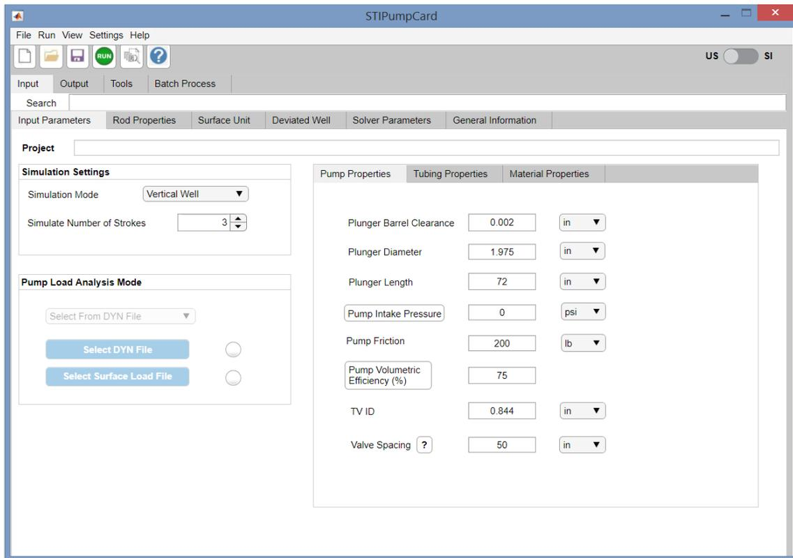
Figure 2 - Input Parameters Panel
