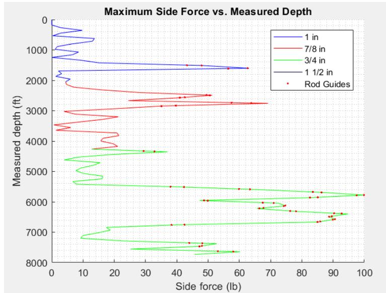
**Figure 44 - Side Force vs. Measured Depth**
