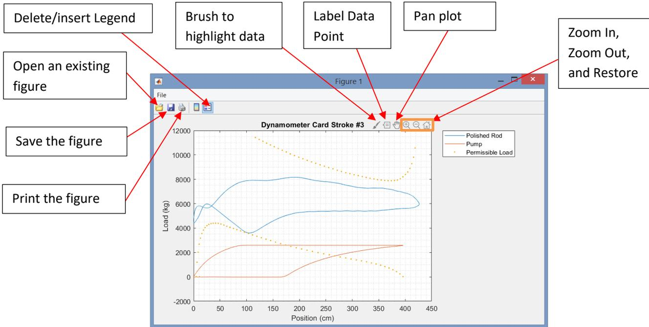
Figure 65 – Interactive figure produced by STIPumpCard
