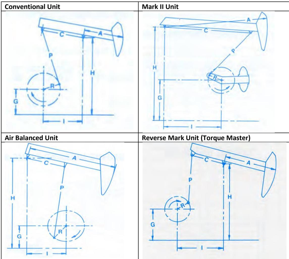
Figure 16 - Beam Balanced Unit Types
