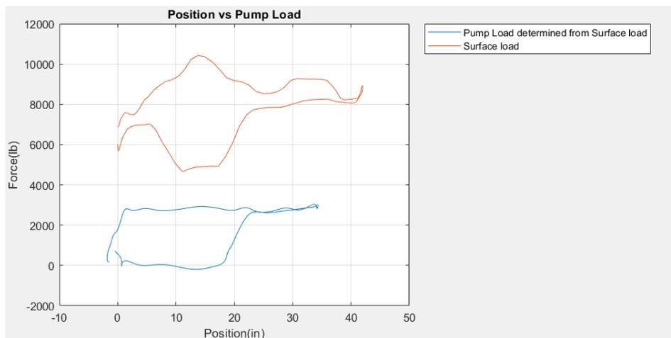
**Figure 48 - Pump Load Analysis Output**
