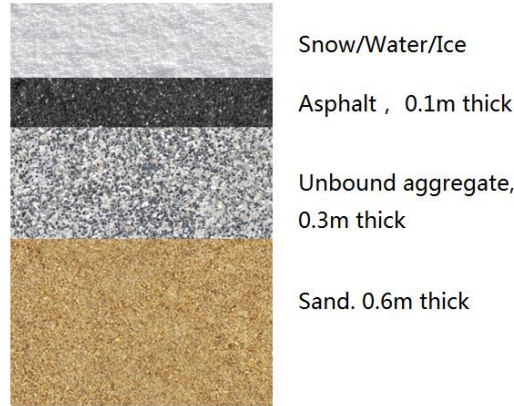
Figure 10 - Typical layers below the ground surface
